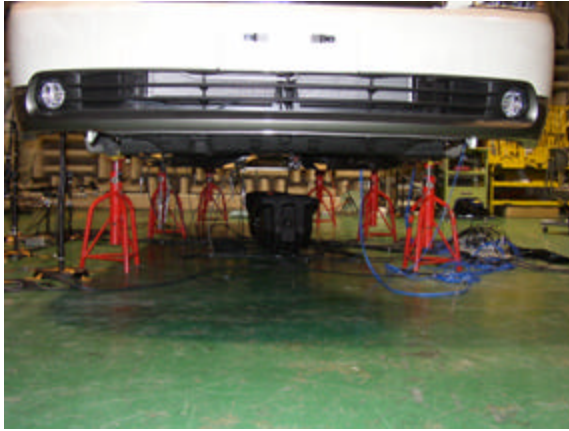
Figure 4: Speakers underneath center of vehicle
