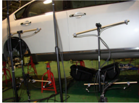
Figure 5: SPL sensor and speaker locations
